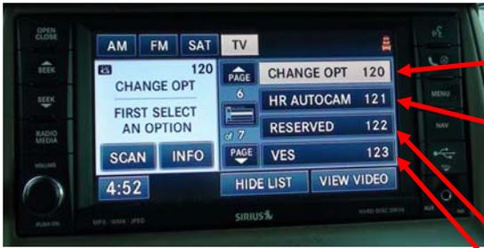
The VES mode is available on the media radio screen view (same HDD, DVD, etc.) Within the VES mode are factory options to send the factory DVD audio and video to an additional screen. A/V output cables are included in your Lockpick radio harness near the white connectors if you would like to use this bonus feature.
